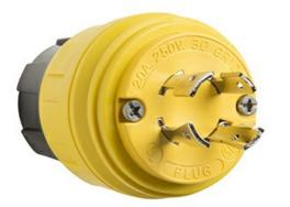
Locking Watertight Plug, 20amp 3 250 volt, NEMA Configuration L15-20, multipoint sealing system provides environmental protection of: NEMA 4, 4X, 6, 6P and IP67 rated.
