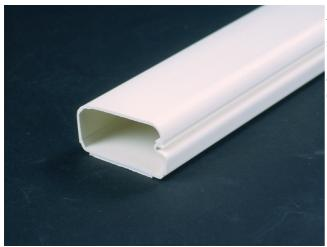
The Uniduct Nonmetallic Latching Raceway System is a one-piece, single channel design, ideally suited to route and protect fiber optic, UTP, and other low-voltage (50V or less) cables in an easy to install and aesthetically pleasing application. 2900 Series Co-extruded design has a smooth plastic finish with adhesive backing. Available in 8ft (2.44m) lengths, packed 160ft (48.8m) per carton.
