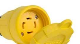
Locking Watertight Connector, 30amp 3 250volt, NEMA Configuration L15-30, multipoint sealing system provides environmental protection of NEMA 4, 4X, 6, 6P, and IP67 rated.
