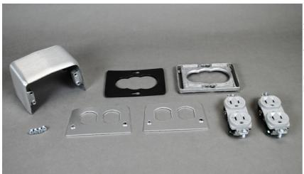
20A 125V duplex plate two sides. 20A 125V Receptacles included. NOTE: Four-piece service fittings include: housing and base plate. Receptacles included when indicated in part number description. 525 Series Service Fittings have 27 cubic inches (442ml) of capacity.
