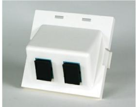
The Series II, Dual, Multimode, SC Simplex, Aqua Adapters (2-Fiber), White Adapter Plate, has two simplex adapters with 180° exit, and ceramic alignment sleeves. This adapter panel is 2 units high. These adapter panels include dust caps, and offers two insests for optional icons (Not Included), to label each connector and indicate its purpose. Compatible With: Series-II Workstation Face Plates and Series-II Workstation Surface Mount Boxes. Wiremold raceway series 2700, 2800, and 2900
