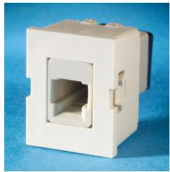
The TracJack, Multimode, MT-RJ Adapter (2-Fiber), White Adapter Plate, has one MT-RJ adapter, with ceramic alignment sleeves, mounted at a 180° exit angle. This adapter panel is 1 unit high. TracJack modules offer flexabilty with structured cabling at the workstation or in furniture with a modular design and a wide variety of connectivity options. Inteligent engineering simplifies and speeds up moves, adds, and changes with a front removeable design. Compatible With: All TracJack faceplates
