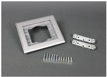
One gang brushed aluminum combination carpet and tile flange, for OmniBox® and Modulink™ Series floor boxes. Flange is 5.940 inch x 4.920 inch (150.9mm x 125.0mm). Accepts Ortronics MAB6TJ TracJack and MAB3S2 Series II, and Wiremold CM Series Open System adapters, sold separately. NOTE: Brushed aluminum flanges come with beveled edges. Brass cover plates can only be used with brass flanges. Brushed aluminum flanges come with beveled edges.
