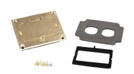
Brass GFI cover plate, for OmniBox® and Modulink™ Series floor boxes. Cover plate is 3.156 inch x 4.182 inch (80.2mm x 106.2mm). May be used with Wiremold CM Series adapters and Ortronics Connectivity Systems in conjunction with 817B, 827B, and 837B Flanges.
