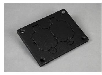
Black powdercoat duplex cover plate, for OmniBox® and Modulink™ Series floor boxes. Cover plate is 3.290 inch x 4.310 inch (83.6mm x 109.5mm). Flip lids can also be used with 106 type frames for communications. NOTE: Brass covers and flanges are not interchangeable with aluminum or nonmetallic covers and flanges. Nonmetallic covers are interchangeable with aluminum flanges.
