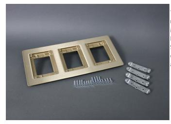
Three gang brass combination carpet and tile flange, for OmniBox® and Modulink<sup>™</sup> Series floor boxes. Flange is 6.080 inch x13.310 inch (154.4mm x 338.1mm). Accepts Ortronics MAB6TJ TracJack and MAB3S2 Series II, and Wiremold CM Series Open System adapters, sold separately. NOTE: Brass cover plates can only be used with brass flanges. Brushed aluminum flanges come with beveled edges.
