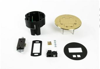
Includes round PVC floor box, one 15A, 125V tamper-resistant decorator style duplex receptacle, one coax F connector, one RJ45 Category 5e connector, and brass duplex opening cover plate with single flip lid.
