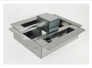
1-Gang Fire Classified Steel Floor Box. Adjustment range over deck of 2" (51mm) minimum to 6-1/2" (165mm) maximum. One 2" (51mm) conduit feed opening. Box Capacity - 53 cubic inches. This box preserves up to a 3-hour fire rating of floors in which it has been installed.
