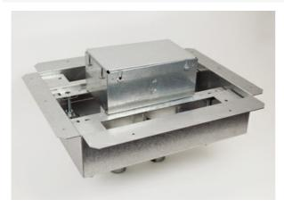
2-Gang Fire Classified Steel Floor Box. Adjustment range over deck of 2" (51mm) minimum to 5" (127mm) maximum. Two 1 1/4" (32mm) conduit feed openings. Box Capacity - 58.5 cubic inches per gang. This floor box preserves the 2-hour fire rating of floors in which it has been installed.
