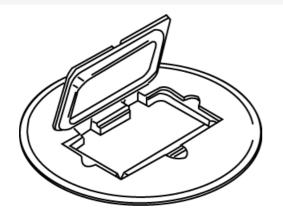
The Wiremold Ratchet-Pro™ brushed aluminum GFI cover plate with decora flip lid, 5 1/2 inch (140mm) for carpet or tile installations. Cover also works with 880 Series™ boxes. NOTE: All cover plates are furnished with gasket and three screws.
