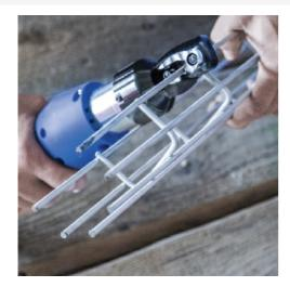
The battery powered wire mesh cable tray cutter is able to cut Steel or Stainless Steel trays up to 6mm dia easily, quickly, and cleanly.
