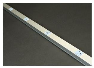
Available in 5' (1.5m) length with 9" spacing. 15A tamper-resistant receptacles. 3-wire, #12 USB Plugmold THHN (1 hot, 1 neutral and insulated ground conductor). .040" (1.0 mm) aluminum housing. Packed two per carton. Each unit supplied with one (1) Coupling and two (2) Blank End Fittings. USB is 2.4 Amps (shared between two ports) 5VDC. Please note the charging load on one module will not affect the charging performance of the other USB modules in the product.
