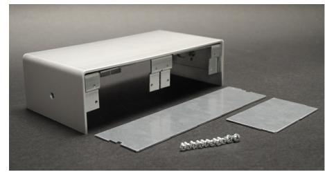
Aluminum housing and base 9 1/4'' x 4 1/2'' x 2 1/2'' (235mm x 114mm x 64mm) are provided with four (4) 1" trade size knockouts in base for hardwiring unit and two dividers which allow units to be divided on either the ''X'' or ''Y'' axis/plane. Accommodates a variety of power (NEMA or decorator), and supports Ortronics and Wiremold Open Systems connectivity. Portals are field configurable by ordering the corresponding faceplates.
