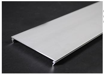
6063-T5 extruded aluminum, satin anodized finish, .075'' (1.9mm) wall thickness. This cover is packed eight 5' (1.5m) lengths per carton.
