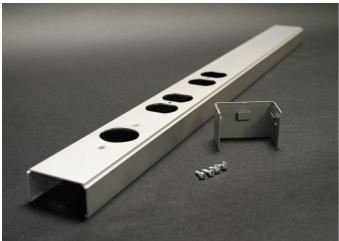
Add power receptacles or devices to existing modular Tele-Power Poles. Includes receptacle mounting bracket. Face diameter of single receptacle: 1.38" - 1.40" (35mm - 36mm). Anodized Aluminum. 1" x 2 1/4" x 28" (25mm x 57mm x 711mm).
