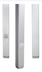
Two-compartment pole. Nominal material thickness .050" [1.8mm]. Length: 10' 5" [3.2m]. Furnished unwired without outlets. Two 8" [203mm] removable covers with KOs for modular jacks and modular furniture communication outlets. Mounting hardware, entrance end plate and ceiling trim plates furnished. NOTE: Custom options - features such as colors or other lengths [20' [6.1m] maximum] available on custom orders.
