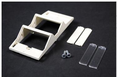
For use with multi-channel raceway device brackets and WallSource device mounting brackets. Angled exit provides additional mounting depth required for A/V connections as well as ensuring the required bend radius for UTP and fiber optic cabling. Holds two Ortronics Series II modules. Fits 5507 Series Faceplate opening. Fits 5507 Series Faceplate opening.
