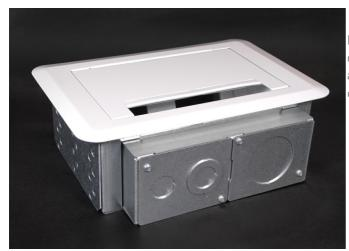
Designed to fit and be concealed behind 42" or larger flat screen displays. Can be installed in both new work and old work applications. Has 4 NEMA size openings for power, communication, or A/V devices.
