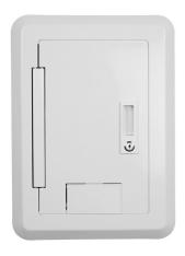
Decorative wall box cover designed to fit onto the 4-gang hinged wall box (EHWB4). Cover comes complete with a hinge that allows the cover to open a full 180 degrees, an integrated handle with lock and key set, and an egress door that allows the cables to exit the box flush against the wall. The cover is offered in two powder-coated finishes white: EHWBC4-WH or black EHWBC4-BK.
