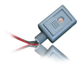
The EM-24A2 and EM-24D2 are low voltage photocells used for controlling exterior lighting. It works with Wattstopper power packs and lighting control panels (Lighting Integrator and LP series panels) by signalling a change in light levels to the panel.
