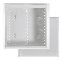
This 14"" On-Q enclosure is the perfect solution for a basic structured wiring system. It features larger top openings that make pulling wire easier as well as additional knockouts, more side lances, and side tabs for more flexible mounting. It includes
