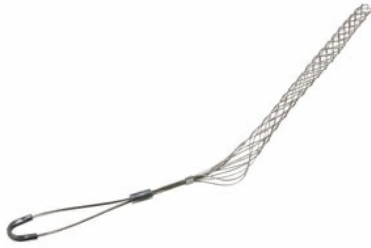
FC075OF: Standard Duty, Closed Mesh, Offset Eye Grips, Cable Diameter 0.75 - 0.99 inches, Bale Length 4-in, Mesh Length 14-in, Break Strength 960 lbs.
