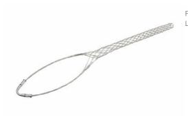
FC075U: Standard Duty, Closed Mesh, Single-Eye Grip, Cable Diameter 0.75 - 0.99 inches, Bale Length 8-in, Mesh Length 14-in, Break Strength 1300 lbs.
