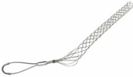
FC1250F: Standard Duty, Closed Mesh, Offset Eye Grips, Cable Diameter 1.25 - 1.49 inches, Bale Length 5-in, Mesh Length 16-in, Break Strength 1680 lbs.
