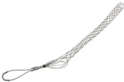
FC1500F: Standard Duty, Closed Mesh, Offset Eye Grips, Cable Diameter 1.50 - 1.74 inches, Bale Length 5-in, Mesh Length 18-in, Break Strength 1680 lbs.
