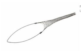
FC250U: Standard Duty, Closed Mesh, Single-Eye Grip, Cable Diameter 2.50 - 2.99 inches, Bale Length 18-in, Mesh Length 24-in, Break Strength 3760 lbs.
