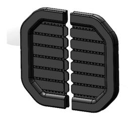
The grommet is designed with 2 half sections for easy installation into any Legrand cabinet with a 4" fan knock-out. Each half contains segmented strips that can be separated to ensure a good seal regardless of the cable bundle size. The strips of each half overlap at the center further ensuring a complete seal.
