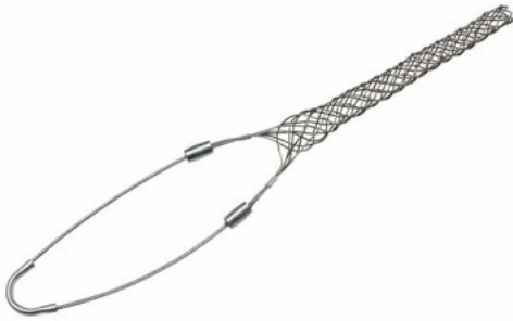
FCSD70: Service Drop, Closed Mesh, Single Eye, Cable Diameter 0.70 - 0.97 inches, Bale Length 8-in, Mesh Length 9-in, Break Strength 1020 lbs.
