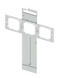
Rough-in is fast and easy with FAS Power. Manufactured floor brackets slide under the sill plate with no vertical measuring needed. Wall brackets with pre-mounted boxes and rings quickly attach to the stud. And for fast job starts, FAS Power products are prepackaged and shipped to the requirements of the contractor. To save time in the planning process, use our online configurator.
