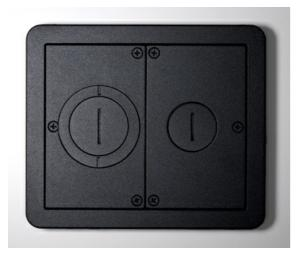
Flanged cover for use in tile or carpet installation. Die-cast aluminum assembly. Provided with one 1in trade size screw plug for power or communication type cabling and one combination 1 1/4in and 2in trade size screw plug for communication type cabling. Allows for feeding both power and communication cabling. NOTE: Add suffix "TR" to the end of the part number to indicate tamper-resistant cover assembly. Tamper-resistant versions are secured with a single tamper-resistant screw.
