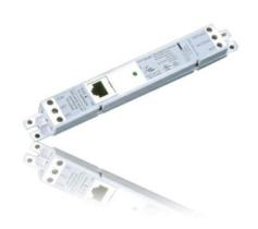
The FS-PP Fixture Power Pack provides 24 VDC operating voltage to the FS Low Voltage Sensor series via the RJ45 connector built onto each sensor. The incorporated Form-C Relay, Normally Open [N/O]/Normally Closed (N/C), can control line or low voltage loads.
