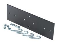
Dimensions: 12 inches H x 7 inches W x .25 inches D Used for junctioning cable runway and equipment racks. Runway can be junctioned parallel or perpendicular to rack. Cable runway mounting brackets mount to the top of the cabinet and provide a surface for attaching 6 in, 12 in, 18 in or 24 in W runway.
