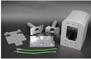
Aluminum housing and side plates, with a steel base and divider, measures 4'' x 5'' x 5 5/8''. Base is configurable to have a combination of two 3/4" knockouts or two 3/4" EMT stubs. Accommodates a variety of power outlets (duplex, decorator, GFCI and up to 30A twist lock). Use Wiremold AVIP to provide communications and A/V. Receptacles and wall plates are sold separately.
