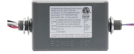
The LDCM-PL-120-277-010V takes a 0-10V dimming signal and a fixed line voltage input and converts it to a reverse phase dimmed output for up to 1000W for a 277V load and 450W for a 120V load. One LDCM-PL can be used per run up to the maximum wattage. The LDCM-PL can be used per run up to the maximum wattage. The LDCM-PL is rated to directly mount to a junction box in a plenum space for easier installations and to meet building requirements.
