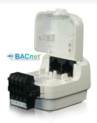
The LMBC-300 Digital Network Bridge provides a segment network connection for a group of Digital Lighting Management (DLM) local network devices. This enables individual DLM local networks to be aggregated into a larger system, which, in turn, can be remotely managed from a DLM Segment Manager or a building automation system (BAS).
