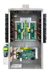
The LMCP series panels are available for Dimming (LMCPx-10V) or Switched(LMCPx) control of lighting and plug loads. The panels can be networked together to enable automation through out an entire facility. The HDR panel relays respond to inputs from Digital Lighting Management (DLM) switches, occupancy sensors, daylight sensors, input modules and 0-10V outputs on dimming panel models.
