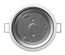
The LMDL-600 is a wireless open loop photo sensor that measures the daylight contribution in order to automatically switch or dim multiple zones of lighting. It is part of the wireless Digital Lighting Management (DLM) system and sends light level signals to control loads connected to DLM on/off or dimming room controllers.
