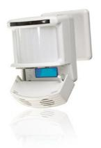
The LMDX-100 Digital Dual Technology Corner Mount Occupancy Sensor uses both passive infrared (PIR) and ultrasonic technologies to achieve precise occupancy sensing for energy-efficient control of lighting and plug loads. It is a digital sensor, and is part of a Wattstopper Digital Lighting Management (DLM) system.
