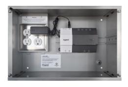
The LMNC-ENC1 is a surface-mount NEMA1-rated enclosure with a DIN rail for mounting one LMJA-8xxx-SM Network Controller with a removable cover. The conduit entrances and enclosure sections for high voltage (Class 1) and low voltage (Class 2) wiring are completely separated.
