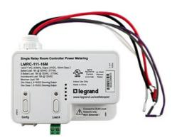
LMRC-111-16M room controllers include one relay capable of switching a 16 amp load, a high-efficiency intelligent switching power supply and both Class 1 and Class 2 0-10 volt outputs for control of dimmable loads including compatible LED drivers or electronic ballasts. Room Controllers are the foundation of a Digital Lighting Management (DLM) system, and allow integration of occupancy sensors, daylighting controls and switches for energyefficient control.
