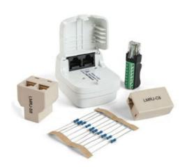
LMRJ series couplers, splitters and other accessories connect Digital Lighting Management (DLM) components without the need for tools or point-to-point discrete wiring. Accessories use preterminated industry standard RJ45 connectors compatible with any RJ45 port on DLM components.
