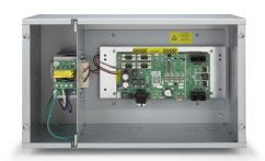
The LMZC-301 zone controller provides power and connectivity to Digital Lighting Management (DLM) fixture controllers as well as switches, occupancy sensors, daylight sensors, and input modules. It is the foundation of a DLM local network for fixture controllers, and includes integral segment network connectivity. The zone controller can be used to enable the automation of lighting functions across a facility.
