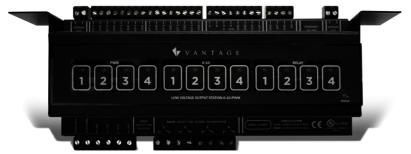
The Low-Voltage Output Station (LVOS) is used for the control and automation of LED, CFL, and CCFL lighting loads requiring either 0-10 or pulse width modulation (PWM) for dimming control. The dry contact inputs can be used with motion sensors, light sensors, pressure sensors, IR inputs, magnetic switches, and more. As part of the Legrand lighting solution, it provides control of LED loads as well as inputs from dry contacts for lighting and automation.
