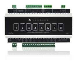
The 0-10 PWM Low-voltage output station (LVOS) is used for the control and automation of LED, CFL, and CCFL lighting loads requiring either 0-10 or PWM for dimming control. The dry contact inputs can be used with motion sensors, light sensors, pressure sensors, IR inputs, magnetic switches, and more. As part of the Vantage lighting solution, it provides control of LED loads as well as inputs from dry contacts for lighting and automation.
