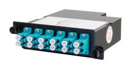
Infinium M4 pre-terminated cassettes with method B provide rapid deployment and have a flipped polarity inside the modules, which use key-up to key-up MPO adapters and allows for straight through patching. The rugged metal housing offers additional durability and includes a built-in internal bend limiting feature to assure optimum optical performance.
