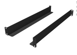
The 6" equipment support brackets can be cantilever mounted at the rear of any Mighty Mo rack and used to support equipment mounted to the front rails. Deeper equipment support brackets are sized to the 16-1/4" to 30" channel racks and 4-point mount with the equipment's mounting ears to provide zero unit support from front to back.
